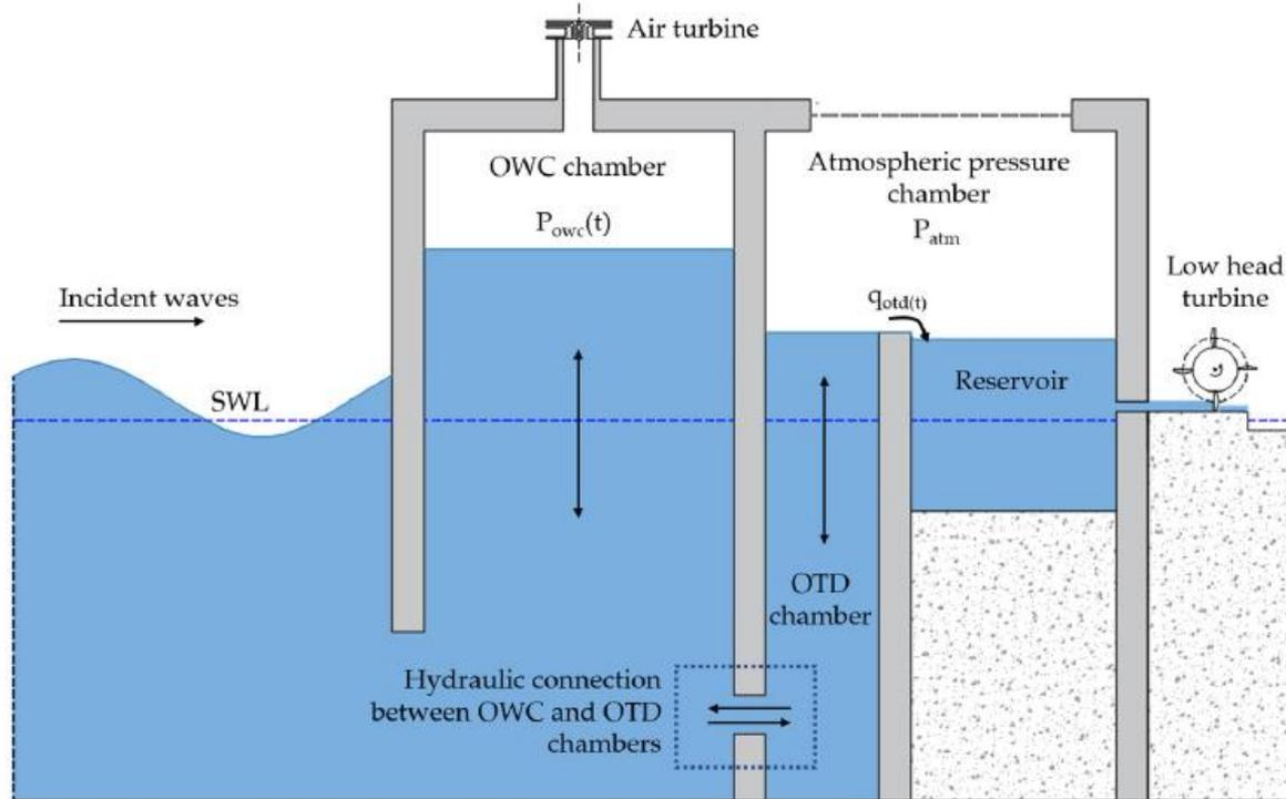
To **reduce** the maximum air pressure in the first chamber (**AVOID DAMAGE**)
