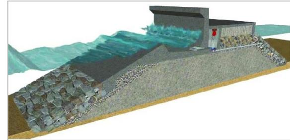
OWC could have limited operability in energetic sea-states (efficiency loss/ **damage at air turbine** for excessive air pressure).
