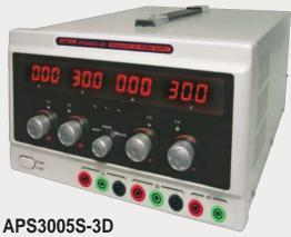
This is a double-channel regulated power supplies with low ripple and noise, reliability. The two channels can be run in series, parallel or in dependently from each other with constant voltage and constant current. There is a 3rd channel which is fixed at 5V and 3 Amps. This unit is designed for use in labs, colleges and in production.
