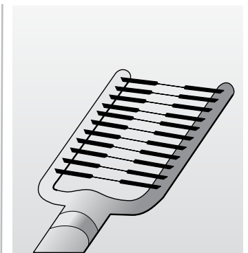
Fig. 18. Wire magazine with 10 wires for gold-plated wire probes.
