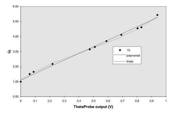
In the range 0 to 1 Volt (corresponding to a soil moisture range 0 to  $\sim$  0.55 by volume), this relationship can be fitted very precisely by a 3rd order polynomial:
