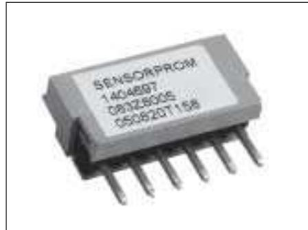
The factory settings matching the sensor are stored in the SENSORPROM® unit. Also customer specified settings are downloaded to the SENSORPROM® unit. Should the signal converter be replaced, the new converter will upload all previous settings and resume measurement without any need for re-programming.
