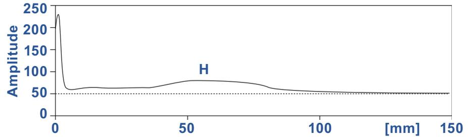
**Broken probe indicated by flat signal around 40 counts**
