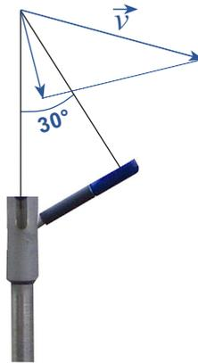
Since the receive beams are slanted at 30°, all three receivers measure the velocity that is slanted about 15° from the transmit beam.
