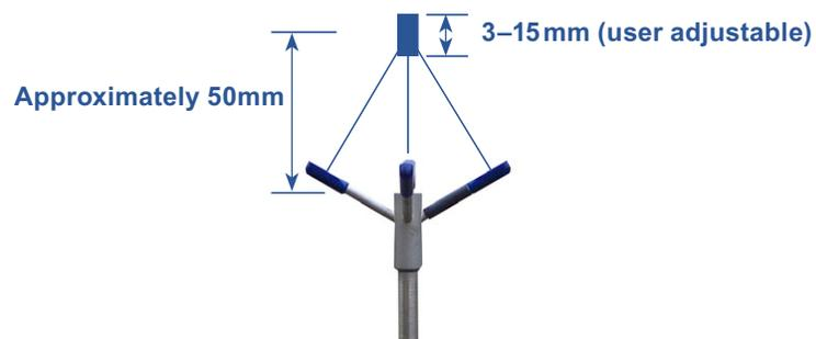
The figure below shows that a transmit/receive beam pair is sensitive to velocity in the direction of the angular bisector between the beams. The arrow indicates a positive velocity.
