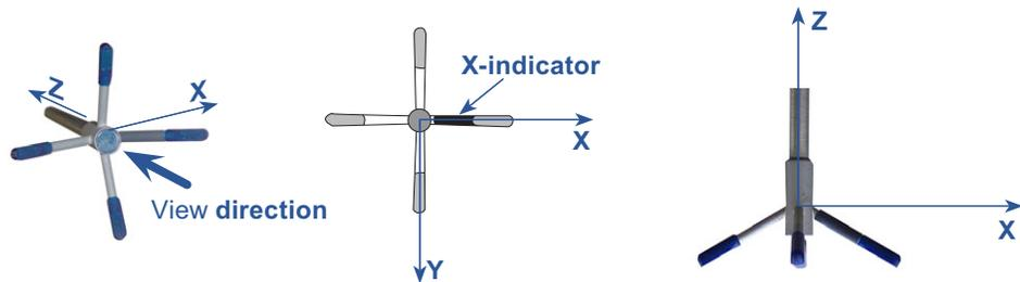
The XYZ coordinates are relative to the probe and independent of whether the Vectrino points up or down.
