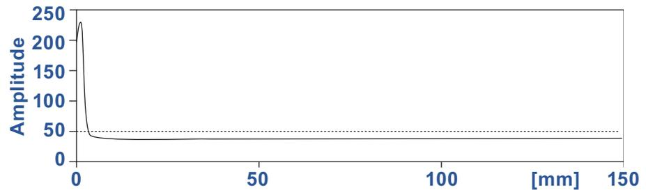
**Weak or non-functioning receive transducer**
