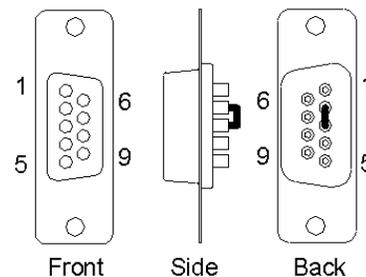
Make a serial loop-back connector by soldering pins 2 and 3 together, as shown
