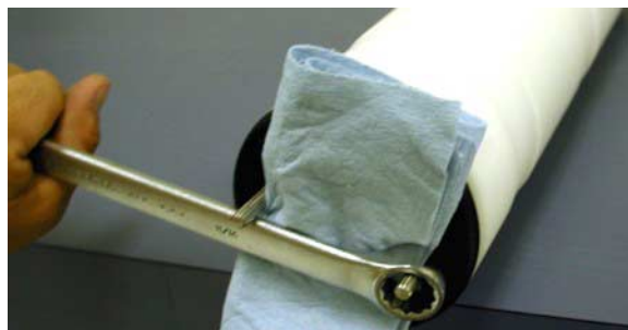
Figure 12 – Triton End Cap Removal
